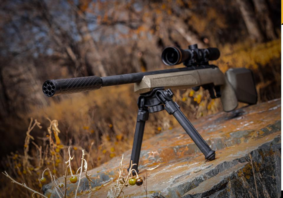
1) Keep your silencer TIGHT! The most common 'death' of a silencer is a Baffle Strike because something wasn't tight or came loose. Both joints must be torqued/tightened before shooting your first shot. Re-torqued after the first shot, and after 5-10 shots, and then periodically. (Front Cap, Suppressor to Firearm). This is particularly important for more powerful firearms.
